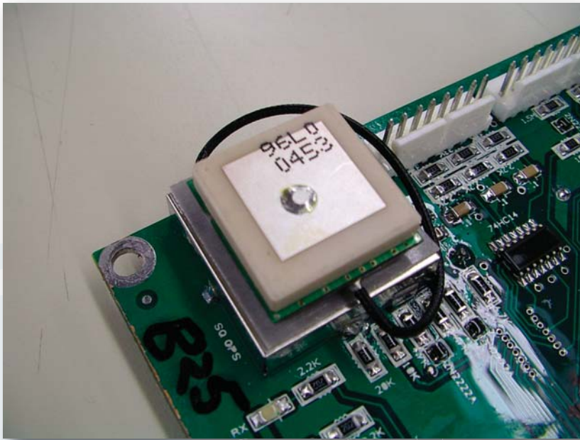
TRIMBLE GPS MODULE WITH WRAPPED ANTENNA
